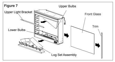
the Log Set contains LED's and wires.
